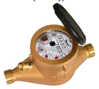
INSA VVS PLUS is IMPELLER (turbine) water meter with magnetic transmission, dry type register for residential application with sizes from Dn15 to Dn50 designed and manufacture by INSA and meets to the requirements of Directive 2014/32/EU on measuring instruments; the European Standard EN14154+A1+A2: Water Meter; the International Organization of Legal Metrology OIML R-49: 2006(E): Water meters intended for the metering of cold potable water and hot water.
