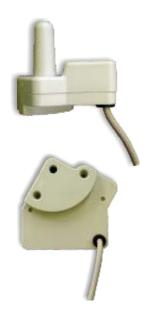
ADO Pulse device is designed for reading residential, industrial and combination water meters. ADO Pulse device has an inductive sensor that counts the rotations of the "liter" pointer and converts the rotations into pulses on the output. ADO Pulse device acts as a reed contact except it does not use a magnet for rotation transmission. Its advantage over the reed contact is that it is impossible to disrupt the inductive sensor by a magnet and therefore the possibility of tampering is eliminated.
