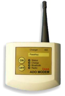
ADO Modem is a device designed for wireless remote reading of ADO module on water meters. The Modem serves as a communication link between the radio modules on the water meters and the handheld terminal.
